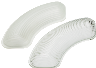
Optics Standard prismatic, borosilicate glass that doesn't fade or degrade. Optional frosted optics provide even greater visual comfort. Injection molded acrylic lens available in wide and narrow.
