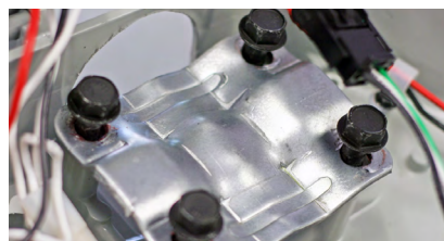
2-bolt mounting on ATB0 & Micro; 4-bolt on ATB2
